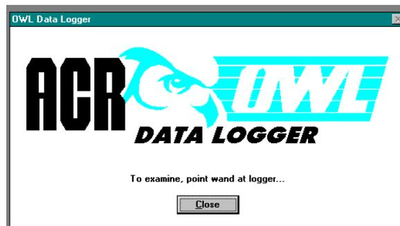
The wand flashes, looking for a logger (the status bar at the bottom left of your screen indicates that TrendReader is scanning for OWL Loggers.) The dialog box asks you to point the wand at the logger to examine the data.
