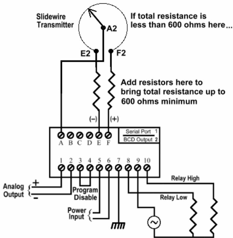
Figure 1.4 Field Wiring Diagram for Low Resistance Transmitters
