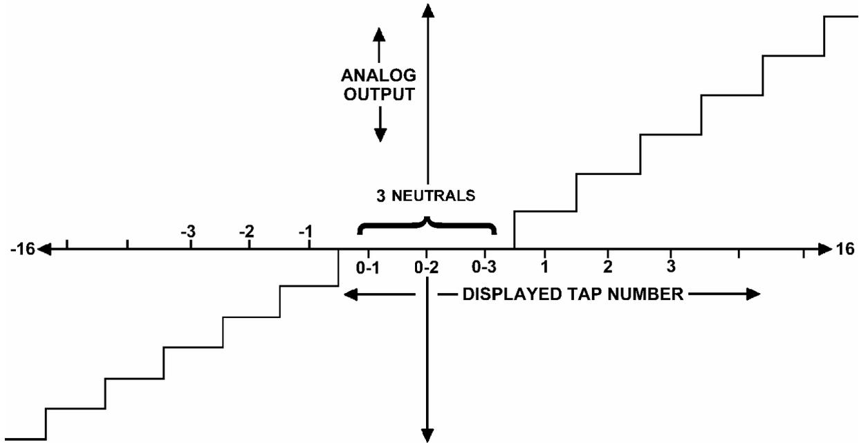
Figure 2.4 Bi-polar Mode Analog Output
