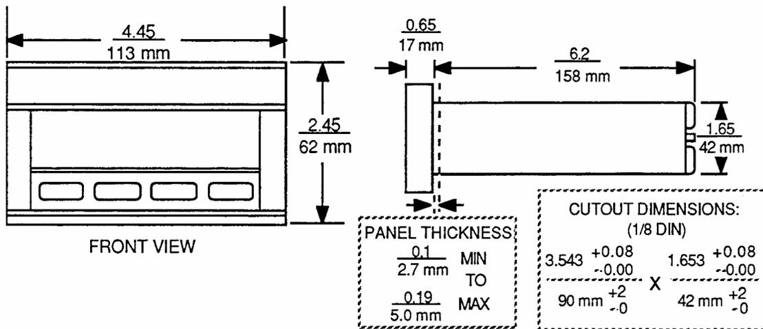
Figure 1.1 Mechanical Dimensions
