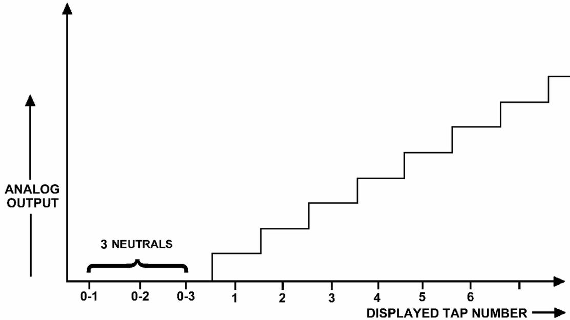
Figure 2.3 Base 0 Uni-polar Mode Analog Output
