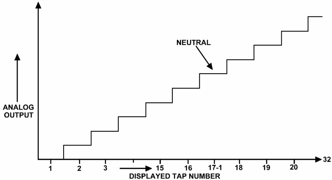
**Figure 2.2 Base 1 Uni-polar Mode Analog Output**
